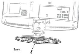
3 Secure the wall mount bracket to the back of your TV using one M4 screw, as indicated in the illustration in Step 1.
